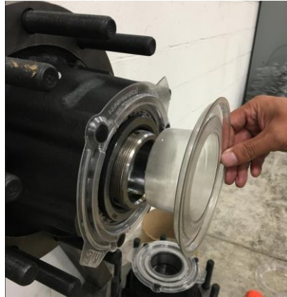
Figure 1. Spindle pushing out outer packaging tube.
